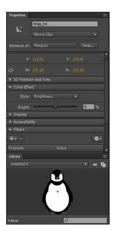
**3** Enter *x* and *y* values for the location of the upper-left corner of the selection. The units are relative to the upper-left corner of the Stage.
