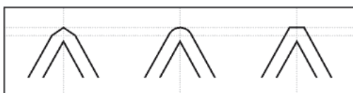
Trap join examples, left to right: miter join, round join, bevel join
