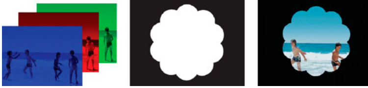
Separated Red, Green, and Blue color channels (left); the alpha channel or mask (center), and all channels viewed together (right)
