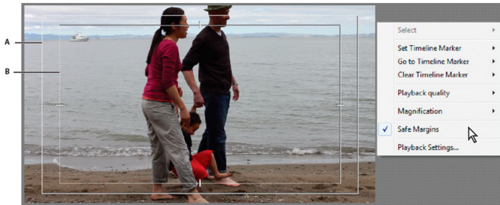
Safe title and safe action margins A Safe title margin B Safe action margin
